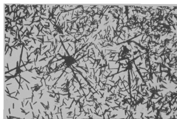
Figure 10. Optical micrographs of SnO 2 /NAF,TTF + electrodes that were cycled 10 times in a 1 M KBr solution and removed from solution in (a) the oxidized form, (b) the reduced form.
